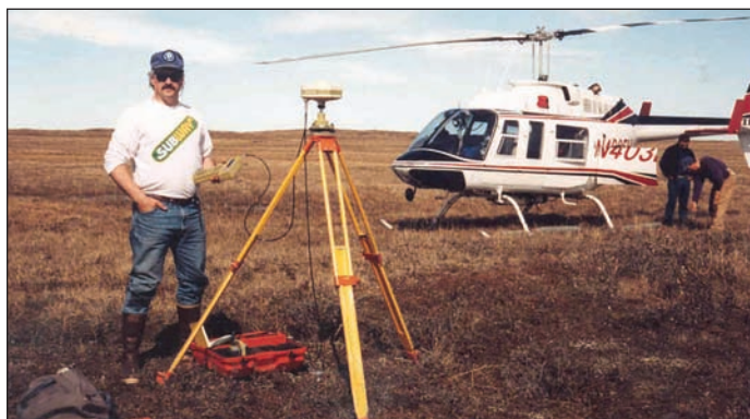
Lounsbury surveyor sets GPS control for Colville River flood plain study (Alpine project 1996)
